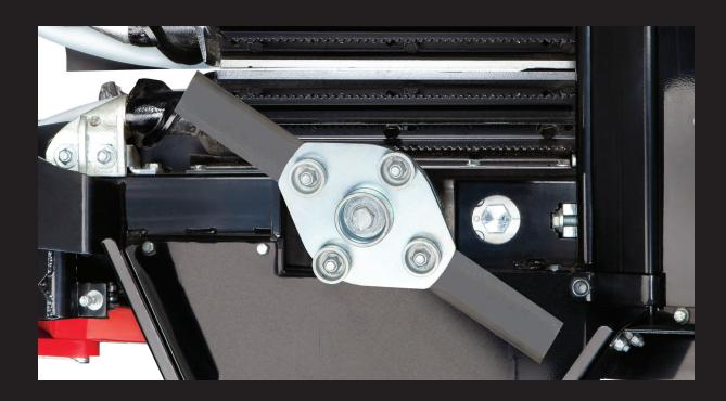
Mounted closer to the front and nearer to the underside of the rolls, MacDon's chopper provides a consistently short residue size. The OctiRoll™ can run closer to the ground to harvest downed corn better and deliver the shortest stubble height possible.
