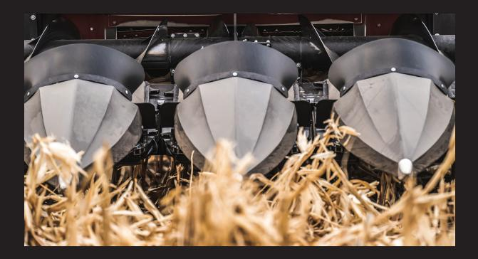
Engineered for efficiency and strength, MacDon's reinforced ribbed snout design reduces drag, guaranteeing a smooth material flow. This distinctive teardrop shape efficiently lifts downed crops, minimizes ear bounce, and skillfully navigates curved rows.
