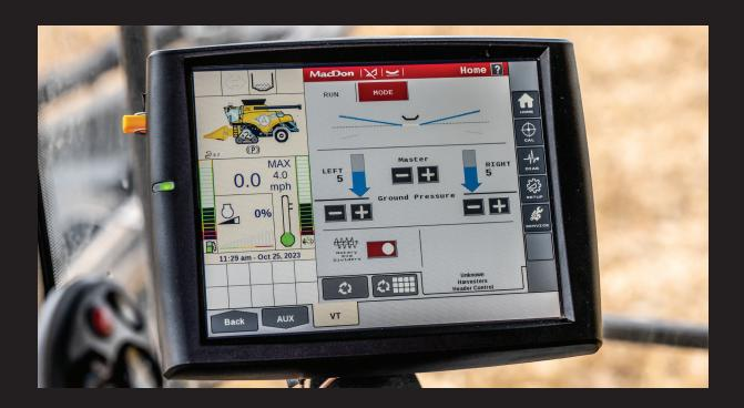
ISOBUS integrated controls mean there is no need for an additional display\*. The user-focused controls provide simple and intuitive header operation; integrated setup, calibration, and diagnostics get you set up and going quickly and easily.
