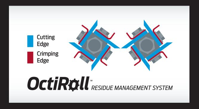
Improving on the traditional snapping roll model, MacDon Corn Headers feature MacDon's innovative OctiRoll™. The unique design of the OctiRoll™ incorporates four point-to-point knives and four serrated edges that alternate to cut and crimp the stalk every 3 inches. The OctiRoll™ cut/crimp action speeds up the microbial breakdown process, helping it decompose quicker than a typical corn header.
