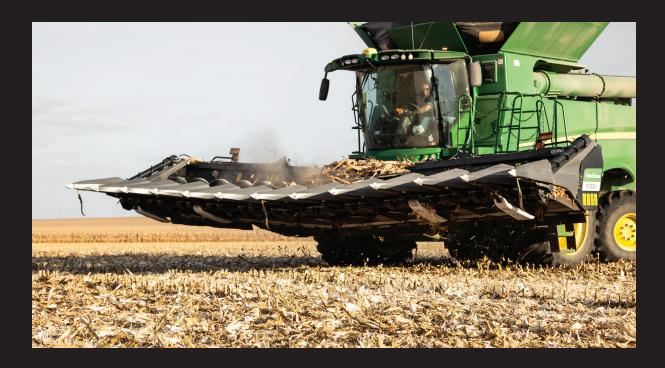
A lightweight yet robust frame and row-unit structure contribute to reducing the overall weight of the header. This reduced frame weight, combined with the high-performance  $OctiRoll^{TM}$ , aluminum gearboxes, and precision choppers, all work together to reduce your overall fuel consumption.
