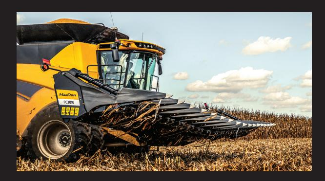
The FlexCorn wings have over 15 degrees of range, so a 16-row header with 30-inch (76.2 cm) spacing provides 61 inches (155 cm) of total flex range on each end.
