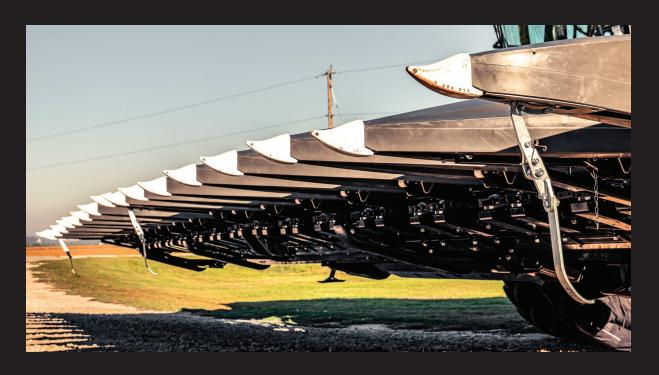
MacDon's AHHC provides automatic height and tilt control to maximize your efficiency in the cornfield. Standard on all FlexCorn and optional on Rigid and Folding Corn Headers. MacDon's AHHC helps increase yield, reduce downtime, and decrease operator fatigue. Paired with MacDon's FluidMotion™ Hydraulic Flex Control, the FlexCorn optimizes header positioning through lift and lateral tilt.
