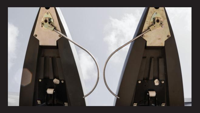
Improving feeding, efficiency, and productivity while reducing operator fatigue, the MacDon Row Guidance System is a great performance option for your MacDon rigid, folding, and flexing corn headers. These two factory-installed and configured metal sensor rods keep you on track all harvest long.
